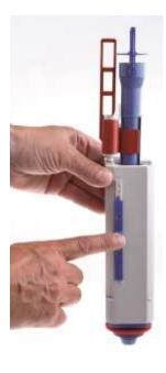
The red pull rod operates the reduced flush, the blue rod the full flush. The valve can be set to a full flush of 4.5, 6 or 9 litres at any time using the slider on the side, while the reduced flush of 3 litres always remains constant.
