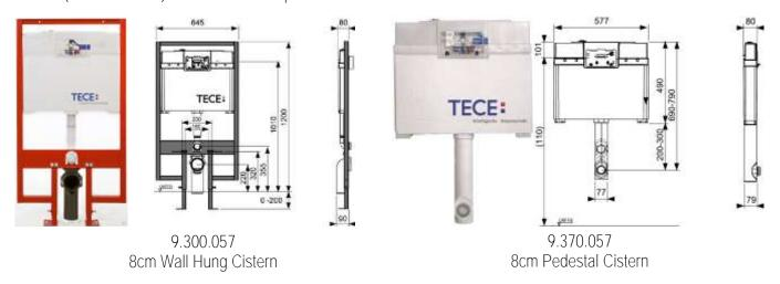
TECEIow Level Suitable for use in minimal hight installation ie. Under a window or vanity height. 18mm non flex board required for standard button installation.
